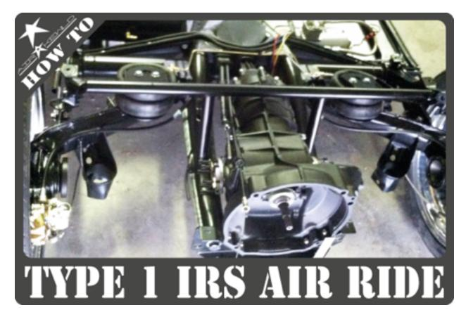
The tutorial is on the installation of a rear Air ride kit for the 1969-1979 US Spec Standard Beetle, Ghia, 1973-74 Type 181 Thing and 1971-79 US Spec Super Beetle
