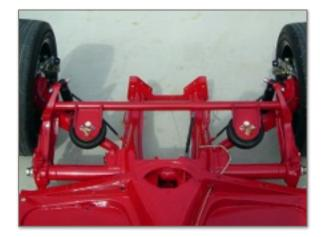
Airbags. Insert the 90 degree push loc fittings into the previously mentioned bushing and the put Teflon tape onto it. Run your lines to a tee and install the inflation stem and pressure test. If you take the time now to leak test them you will not have problems in the future. Take a soapy solution and spray around the fittings to see if you have a leak and fix accordingly.
